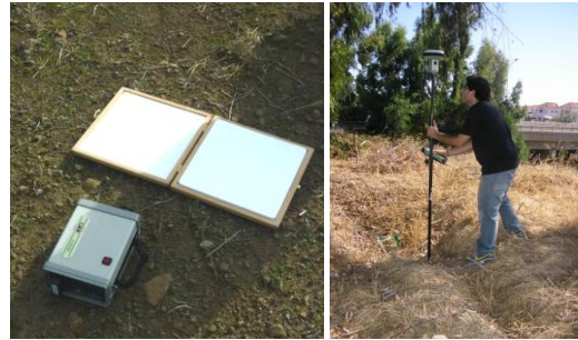
Figure 3. The GER 1500 spectroradiometer used for the collection of ground measurements (left) and the GNSS used for mapping the pipeline (right).
