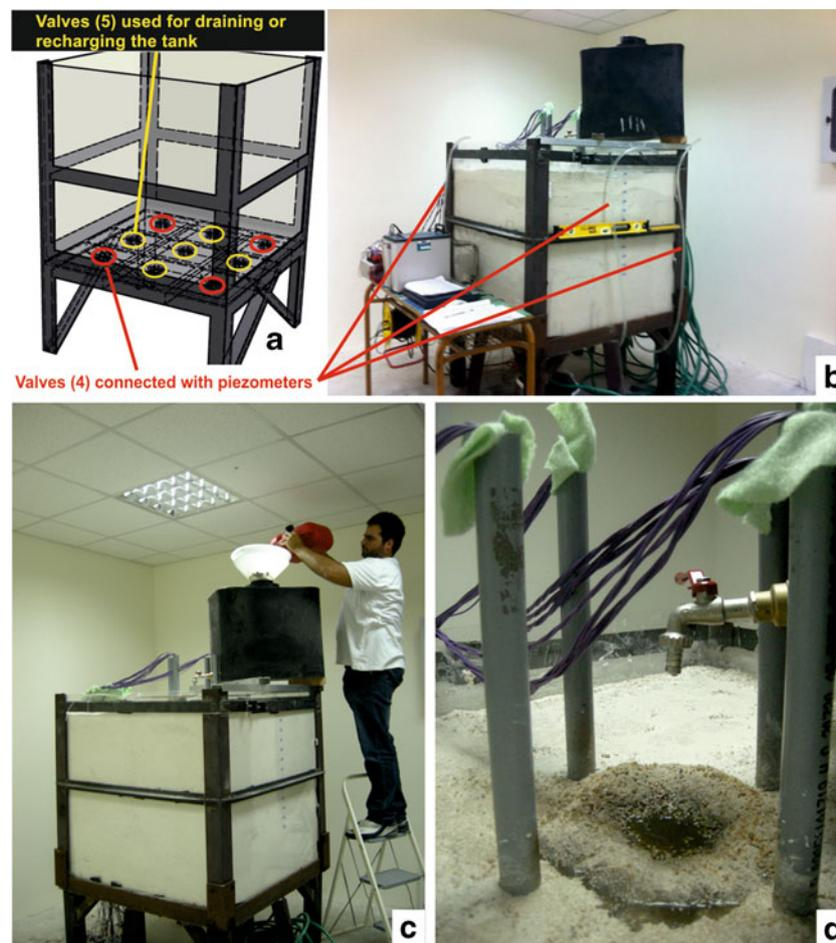
**Fig. 1** a Sketch of the tank before construction and the valves designed at the bottom of the tank for different uses. b Piezometers used for controlling the water table. c Preparation of the container with OOMW before the initialization of the experiment. d Two different flow rates were used in order to simulate the annual deposition of the contaminant. The different flow rate values were used for the FEFLOW simulation
