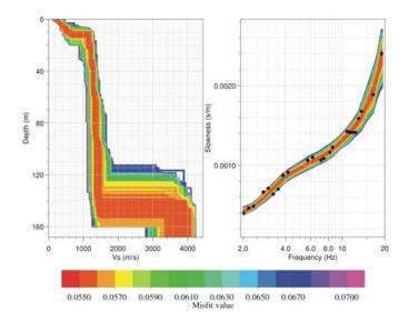
**Fig. 6.** One-dimensional model of shear wave velocity behavior with depth (left) and the corresponding dispersion curves (right). The dark circles present the results of the F-k processing.
