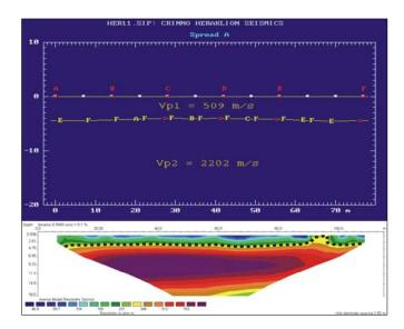
**Fig. 4.** Comparison of the resulted tomographic images from refraction seismics (upper) and geoelectrical tomography (lower) for the same HER11 location.
