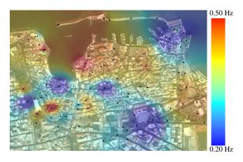
**Fig. 7.** Map of the fundamental eigen-frequencies in the area of Chania.
