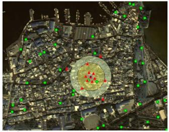
**Fig. 5**. The layout of the microtremor array measurements for the city of Chania. Measurements were carried out within the historical center of the city, between the Venetian fortification walls and the port.
