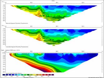
Fig. 2. Electric Resistivity Tomography at site RETH 05.
