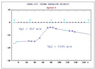
**Fig. 3.** Resulted geophysical structure for SITE02 in Herakleion city.
