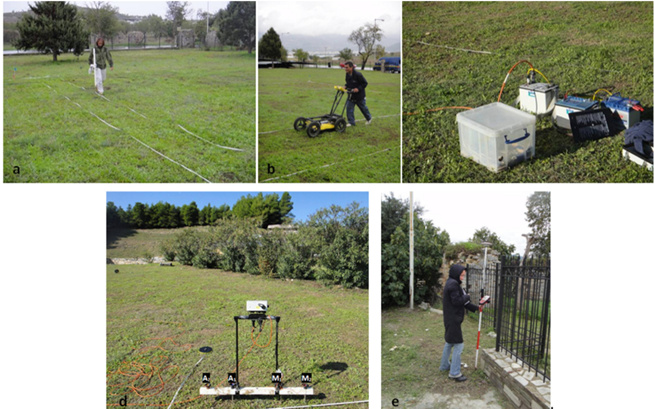
Figure 2. Details of the geophysical survey in the theatre of Demetriada with the magnetic gradiometry (a), the GPR (b), the ERT (c), the multiplexed resistance (d) and the GPS (e).
