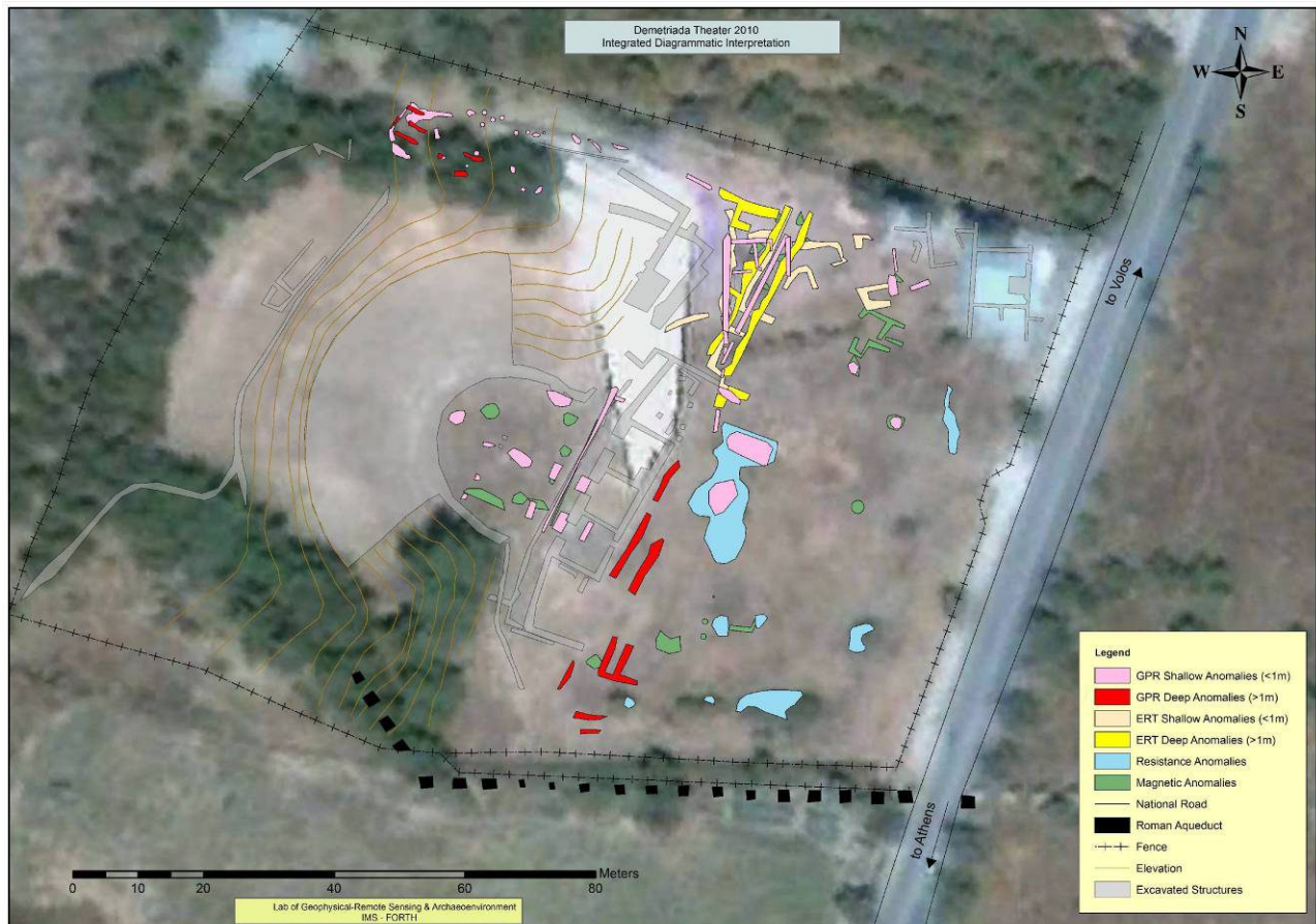
Figure 7. Combined diagrammatic interpretation of the geophysical anomalies indicated by the different methods that applied in the survey of the theatre of Demetriada.
