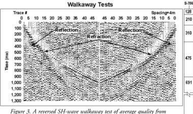
rigure 5. A reversed SH-wave walkaway test of average quality from northeastern Arkansas. The interpreted depth-velocity model (in m/s) for the site is shown at the right. The shear wave velocity of the deeper sediment (below approximately 100m) was not sampled. The 846m depth to bedrock (shaded) was determined by P-wave soundings.
