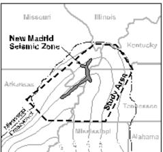
Figure 1. The study area in relation to the Mississippi Embayment and New Madrid Seismic Zone. The poorly consolidated sediments are in excess of 1 km in some parts of the study area.
