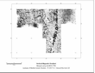
Figure 2. Vertical magnetic gradient grids merged using the GridKnit™ Suturing technique.
