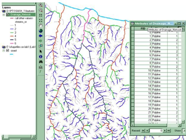
**Figure 10.** Detail of the ordering (according to Strahler's system) of the digitized drainage network originated from the 1:20000 hydrological maps of the study area.
