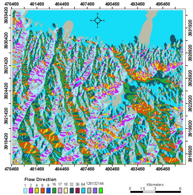
**Figure 8.** Flow direction map which derived from the DEM of the broader Chania area.
