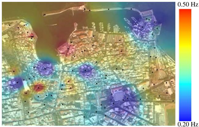
**Fig. 7.** Map of the fundamental eigen-frequencies in the area of Chania.
